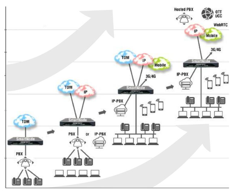
Patton's SmartNode units are available to support any level of integration or dis-integration at the customer premise. SmartNode offers cost-effective and efficient solutions for service providers that save money, reduce hardware requirements, and simplify network architecture at the customer premise. The graphic below shows a schema of the options. The "1-box solution" integrates as many functions as possible into a single device, which we call an Integrated Access Device (IAD).
